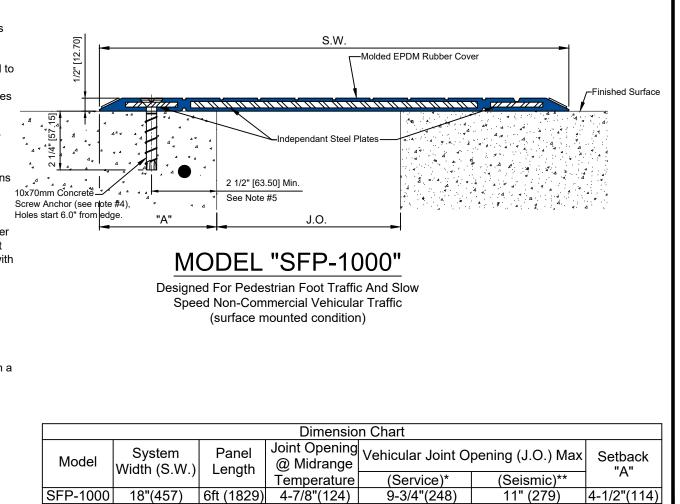
\* Service movements occur due to the following design conditions, including but not limited to, thermal, wind sway, creep and shrinkage.
