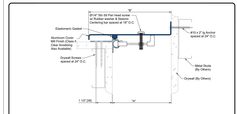
WFI-1000C Thru WFI-2400C DETAIL WALL-TO-CORNER INTERIOR CONDITION
