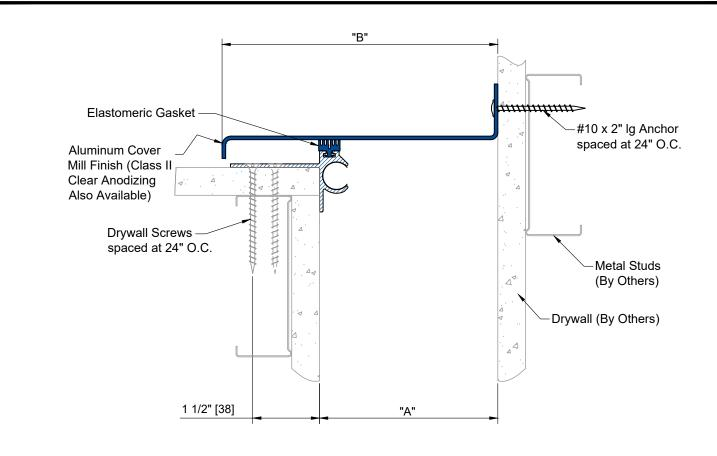
WFI-200C Thru WFI-800C DETAIL WALL-TO-CORNER INTERIOR CONDITION () - Denotes Millimeters
