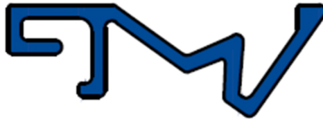
Aluminum wall mount extrusion, P/n: 11206 (Corner Condition)
