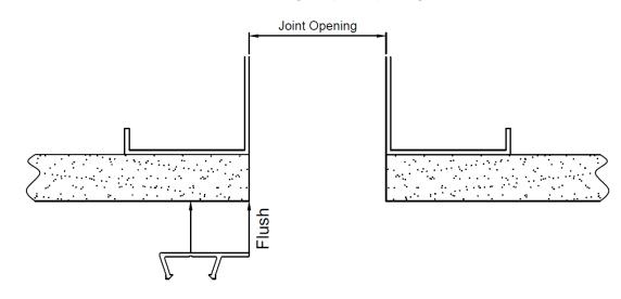
Align and drive drywall screw through base extrusion into wall construction at the specified anchor spacing.
