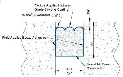
Movement Capability: WBAsics™ Horizontal Foam Seal can accommodate +60% / -60% movement of the joint opening.
