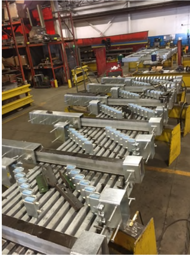
Figure 6: Equidistance springs installed, support bars ready to be strapped on with yokes
